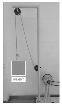
Fig 5: Rope, drum and load arrangement
