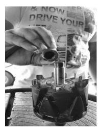
Fig 8: Field of an alternator
